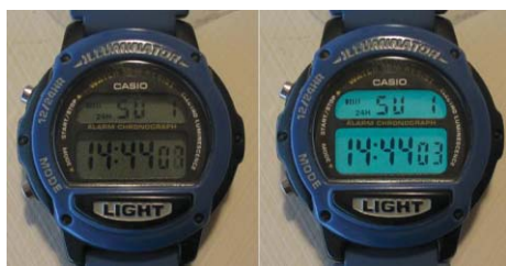
Fig. 1 Application of electroluminescence in lighting up the display in this watch. An electric signal, caused by pressing the 'light' button on the watch, excites the molecules in the display medium that cause luminescence upon their relaxation.
