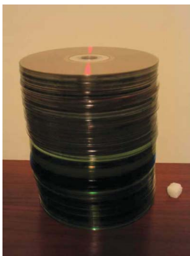
Fig. 3 A photo of 100 stacked DVDs and a sugar cube. If holographic storage lives up to its hype, one will be able to store a terabyte (1000 Gb) of data in a crystal the size of a sugar cube. Employing current commercial optical storage devices, a terabyte of data would fill more than 1000 compact disks, or over a 100 DVDs. The use of an actual sugar cube as a placebo here is a deliberate attempt to emphasise the fact that whilst the optical technology is developing rapidly, scientists are still struggling to find suitable materials for the application.
